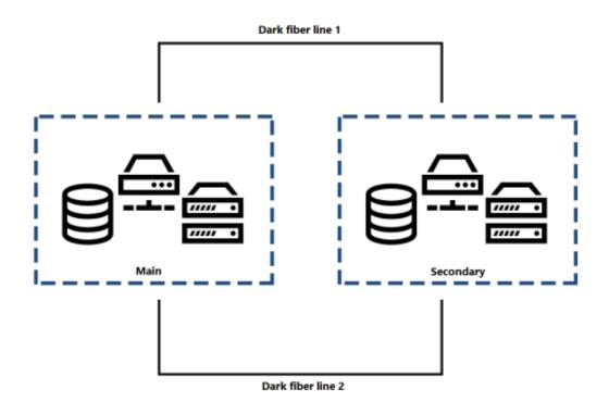
The preservation system is distributed across two physical data centers in active – standby topology. All VM's hosting the components of the preservation system are backed up on a daily basis with a retention period of 30 days, as follows:
